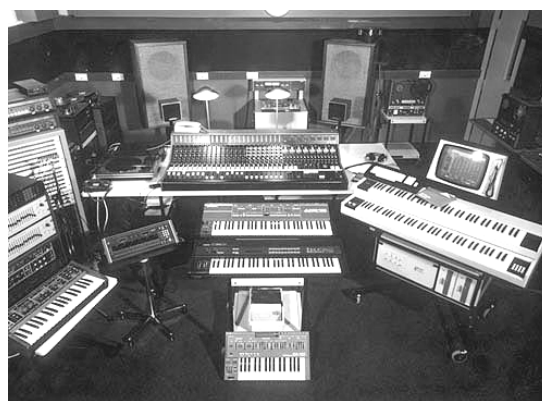
Figure 1: EMS Control Room (later, the Multichannel Studio) in the 1980s. Chilton 24.8.2 desk (middle), Publison DHM89 digital delay/pitch shifter (bottom left), Fairlight CMI series II (right).
