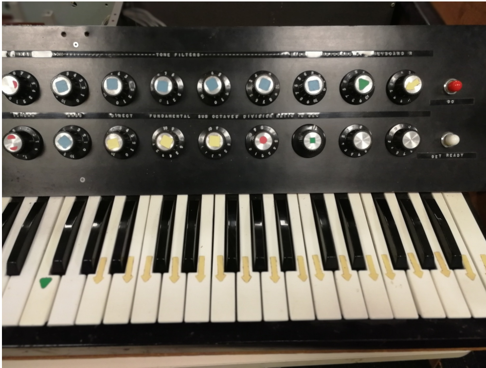
Figure 16 Middle/right section of base unit. Blue and yellow sticker knobs appear to relate to as yet unknown EQ/Filtering circuits/signal processing. Top row last 2 knobs are for left/right keyboard tuning. Furthest right show the ready/go cue light buttons
