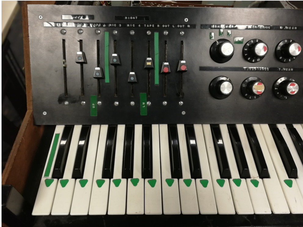
Figure 15 Base Unit left hand section showing mixer and Random voltage/trigger pots (red sticker)
