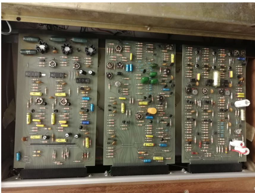
Figure 13 VCS3 R with rear cover removed. No visible modifications to the 3 main boards A, B and C
