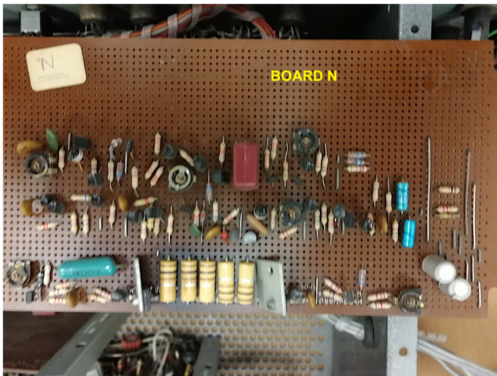
Figure 29 pcb labelled 'N'. Testing shows this is the random voltage/random triggering circuit
