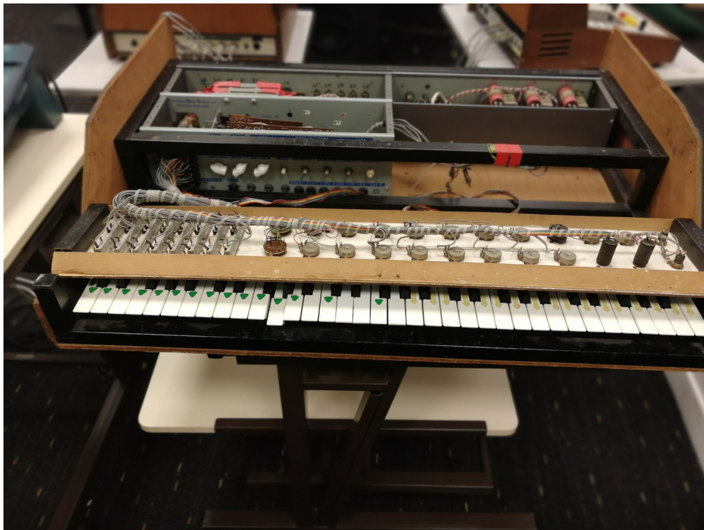
Figure 17 Rear of front panel showing wiring looms from keyboard and the various pots and switches
