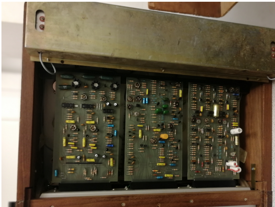
Figure 8 VCS3 L rear cover removed. No visible modifications to pcbs A,B and C
